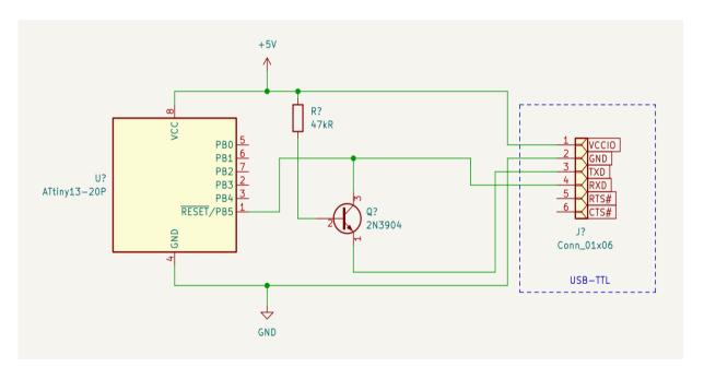
The VCC and GND outputs of the adapter should be connected to the corresponding VCC and GND pins of the microcontroller. The RXD output should be connected to the RESET pin through a 47 k $\Omega$  pull-up resistor, while the TXD output should be connected to the RESET pin through a 2N3904 transistor. The connection circuit (for example, with an
