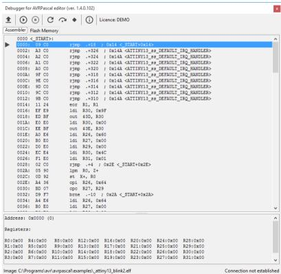
The *Flash Memory* tab displays the loaded flash memory image, differentiating code (blue background) and data (green background) sections. You can view memory bytes in either hexadecimal mode or as ASCII characters.
