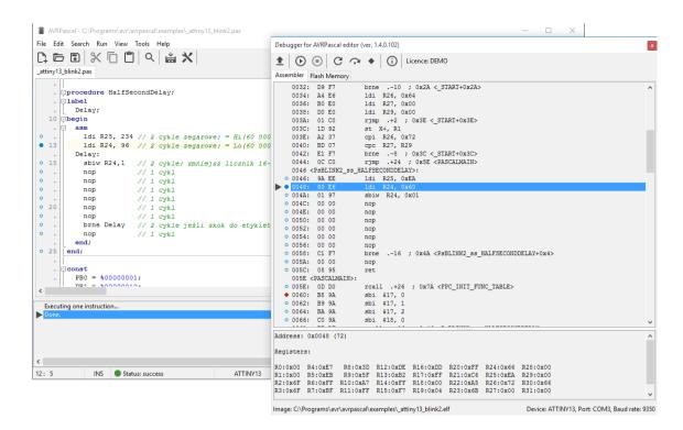
The *Reset* tool is used to reset the microcontroller and return the program execution point to the beginning of the flash memory. In each case, the current content of the microcontroller registers is displayed in the lower panel of the Assembler tab. Finally, the *Config data* function shows the values of the microcontroller's fuse bits.
